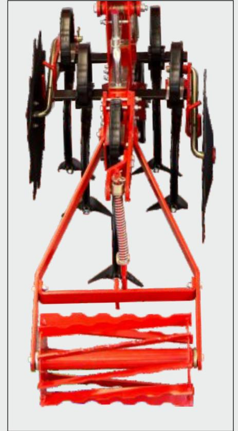
The spacing between the individual working units can be changed easily by loosening the screws that connect the main frame of the machine with the working units.
