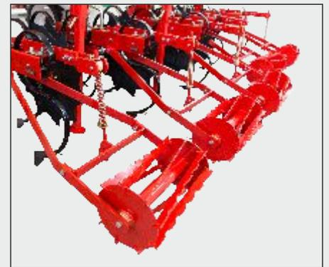
The rear roller provide to crumbling the soil and smooth soil surface.
