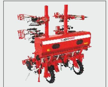
Interrow cultivators are equipped with foldable wings that can be folded in transport position within 2.5m.
